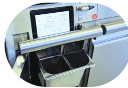
Basin for draining the cooked product into the tank. Guaranteed cleanliness of the station and ease in transporting products.
